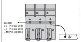
Multiple product installation, busbar E-3, E-5 or E-10 can be used to combine all the earth terminals to earth.
